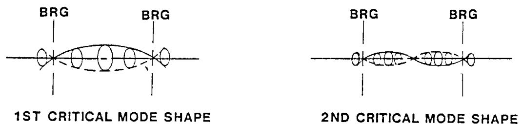
FIGURE 4.39 Rotor lateral critical speed mode shapes: left) 1st critical mode shape, right) 2nd critical mode shape.
