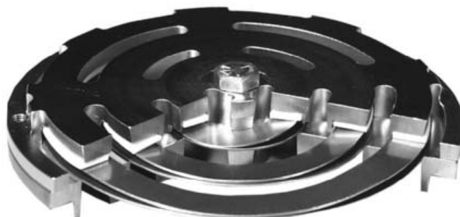
FIGURE 20.2 Ring valve with wafer springs.
