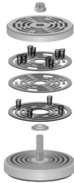
FIGURE 20.5 Double damped valve.
