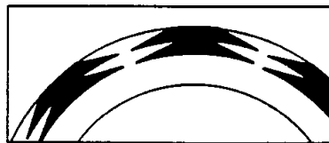
FIGURE 16.17 Bi-directional grooved seal face (John Crane Inc.).
