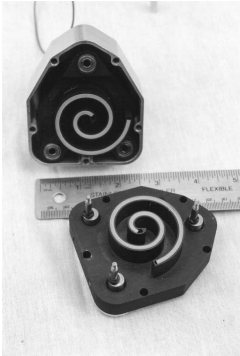
FIGURE 12.4 Typical scroll showing idler shafts.
