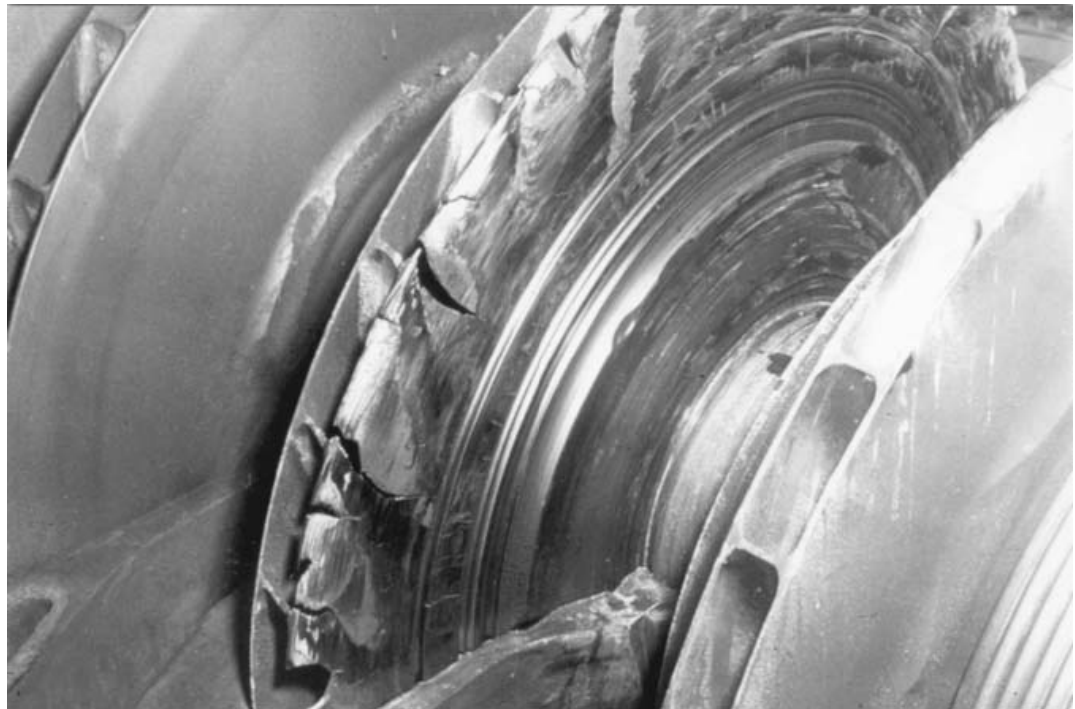
FIGURE 4.53 Damage from surging.
