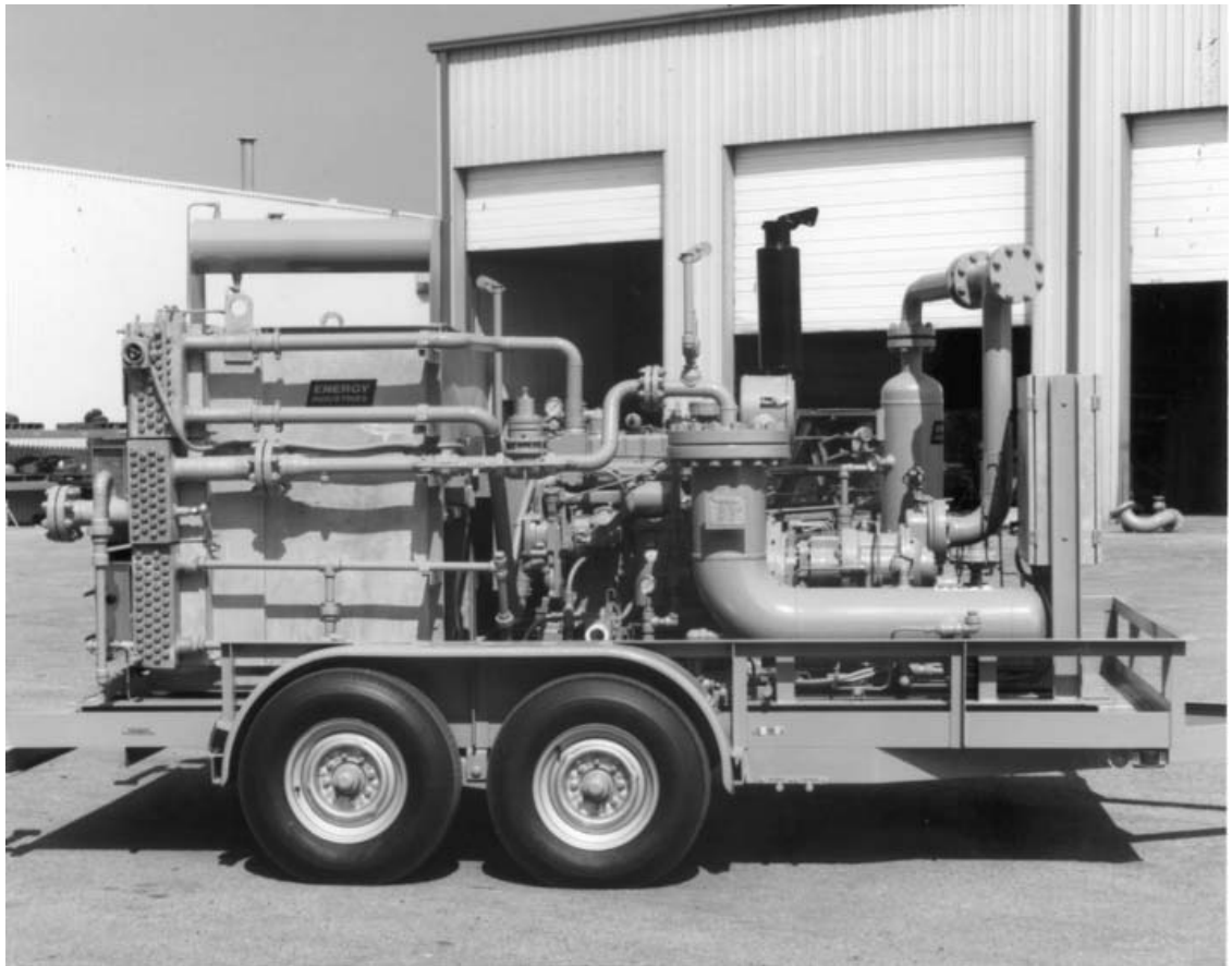
FIGURE 23.10 Trailer-mounted CAT G3304NA/C12 sullair unit.
